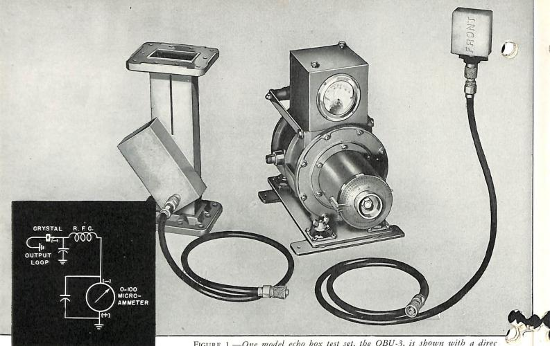
FIGURE 2.-Schematic diagram of the echo box.
