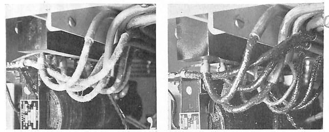
TBM-10 Modulator Unit before and after tropicalization. Note that all cloth covered wires to the modulator transformer T-405 have been attacked by fungus growth.
