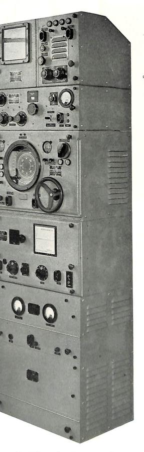
Forward torpedo room sonar stack
