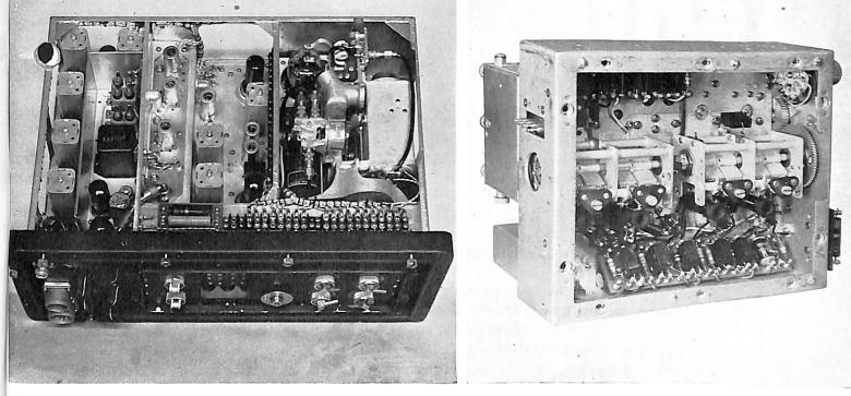
Compact, miniature construction packs a lot of radio in a small package in the Model MAR.
