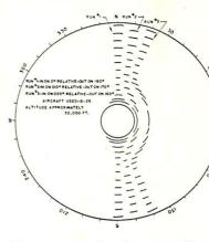
Drawing made from a Zenith-Watch Scope showing the presentation of three different plane runs. The first run passed directly overhead; in the other two the plane passed the antenna to starboard.
