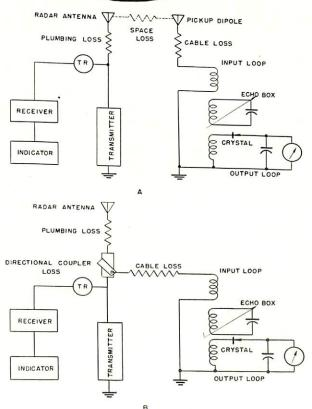
FIGURE 5.—Two methods of feeding the echo box are illustrated above. Note that when the directional coupler is used, the plumbing loss is not present.
