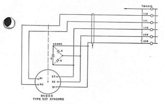
FIGURE 3.—Field Change No. 5. Compensating capacitors are added in the conventional manner.
