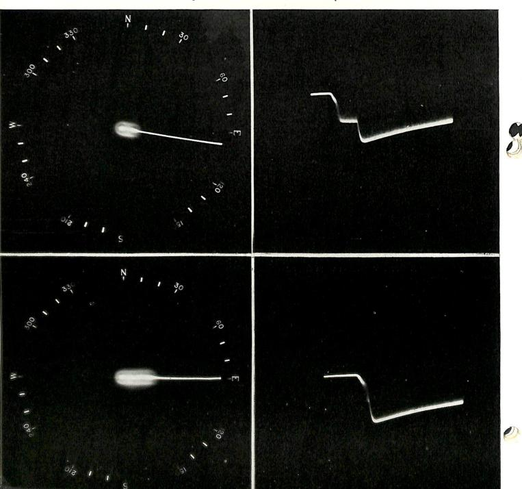
a. With antenna rotating, set the receiver gain at a minimum and adjust the intensity so that a very slight radial trace appears on the scope.
