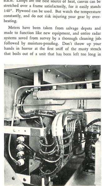
Right side of bottom deck of a TBM-10 Modulator Unit before and after the tropicalization treatment. This is new equipment being unpacked and treated before going into service with the fleet.
