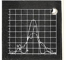
echo box when the echo box is tuned to the maximum of the spectrum. If the pulse length is long, the spectrum curve is consequently high and narrow, and the meter reading high. Where the pulse length is shorter the spectrum curve is flatter and the meter reading will be lower.
